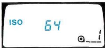
3. Turn either control dial until the desired film speed setting appears in the body data panel.
