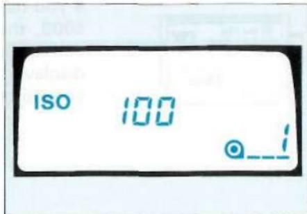
3. Close the back cover and move the main switch to ON. The camera will automatically advance the film to the first frame and 1 will appear in the film counter.
