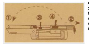
Open the lighter body (1) by pushing the tab on the bottom. Slide (2) moves out. If the flint (3) looks worn, you may try to turn it over so that the unused portion of the flint is against the striker wheel to extend its life, or replace it. (4) is room for spare flints. If the flint gets stuck, use a small needle to remove it.
