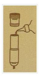
Pull the fuel chamber downward, out of its casing. Hold with wick side down and pull the cap off. Slowly fill the cotton-filled fuel chamber with fluid until approximately three drops of fluid fall from the wick. Replace the cap and return the fuel chamber to its casing.
