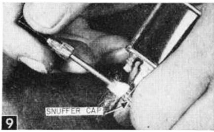
Wipe inside of snuffer cap with pipe cleaner or small screwdriver wound with cotton. Drop a now flint into flint cap opening, insert pressure spring and then screw in the flint cap.
