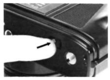
1. To rewind the film, remove the camera's case if on, then press the rewind release on the camera bottom.
