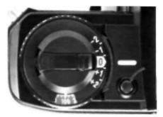
To deliberately increase or decrease exposure from the normal metered value, turn the exposure-adjustment control while pressing the lock release until the desired position is aligned with the index. Set minus (—) numbers to darken exposure and plus (+) numbers to lighten exposure, as indicated in the table.
