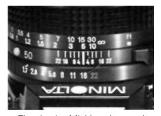
The depth-of-field scale can also be used to zone focus, i.e., set the focusing ring so that some anticipated action will take place within the limits of the depth of field. For example, if you want any subject within a range of 2.6m (approx. 8-1/2 ft.) to infinity to be reasonably sharp and the lighting conditions allow you to set an aperture of f/16 in A or M mode with a 50mm f/1.7 lens, set the lens so the infinity mark is opposite the "16" on the right end of the scale.
