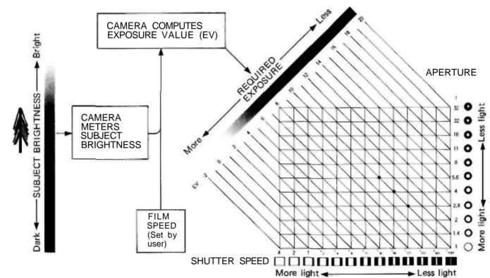
When you take a picture, light from the subject passes through the lens and open shutter, striking the film to form an image. To obtain correct exposure for the subject's brightness and film being used, the aperture (size of the diaphragm opening) and shutter speed (length of time the shutter curtain is kept open) must be controlled.
