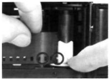
3. Pull out enough film leader to just reach the take-up spool, then insert the end into a slot on the left (as shown above), making sure it does not protrude from another slot. A hole in the film should be lined up with the tooth on the take-up spool, and the sprocket teeth should be engaged with holes at the bottom of the film.
