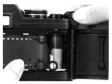
4. With the film held against the sprocket by your left hand, slowly operate the film-advance lever until the film is wound firmly around the take-up spool, the sprocket teeth are engaged with holes on both edges of the film, and the slack in the film is taken up.
