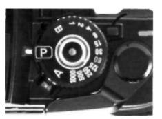
Mode/shutter-speed selector and P/A-lock release
