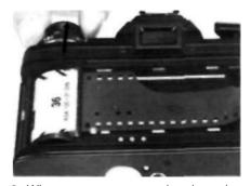
3. When you are certain that the exposed film is completely rewound into the cartridge, pull up on the back-cover release knob to open the back, then remove the cartridge.
