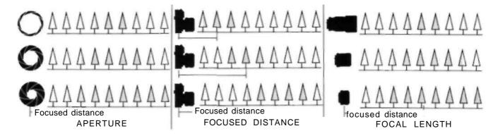
The range behind and in front of the focused distance within which the image appears acceptably sharp is called the depth of field.
