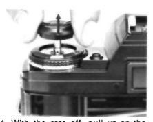
1. With the case off, pull up on the back-cover release knob until the camera back springs open. Gently blow away any dust or other particles inside with a blower brush.
