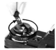
2. Unfold the rewind crank and turn it in the direction of the arrow until the red bar in the Safe Load Signal moves out of the window to the left. Near the end you will feel tension on the film increase then completely disappear, and the crank will then turn freely.
