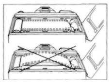
5. After making sure the film is taut, close the camera back by pushing in on it until it clicks shut. A red "S" should now appear opposite the index in the frame counter.
