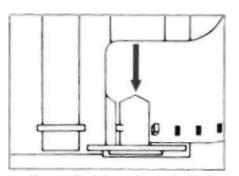
If you find it easier to hold the film leader in your right hand, insert the film as shown in the diagram above, making sure the take-up spool tooth is properly engaged with a hole.
