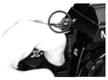
To obtain proper exposure in high-contrast lighting situations where your subject is on the edge of the frame or occupies only a small portion in the center, use the AE lock as follows:
