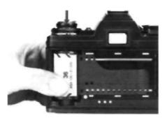
2. Leaving the knob pulled out, position a 35mm film cartridge as shown with the projecting spool down. Then push the knob all the way in, rotating it slightly if necessary.
