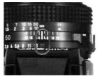
Set and lock lens at minimum aperture (green figure).
